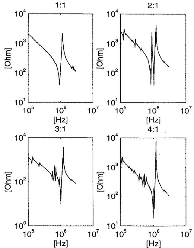
Figure 2: Electrical impedance magnitude of parallelpipeds of elevation height to width aspect ratios of 1:1 to 4:1. The thickness to width aspect ratio in each case is 2:1.
