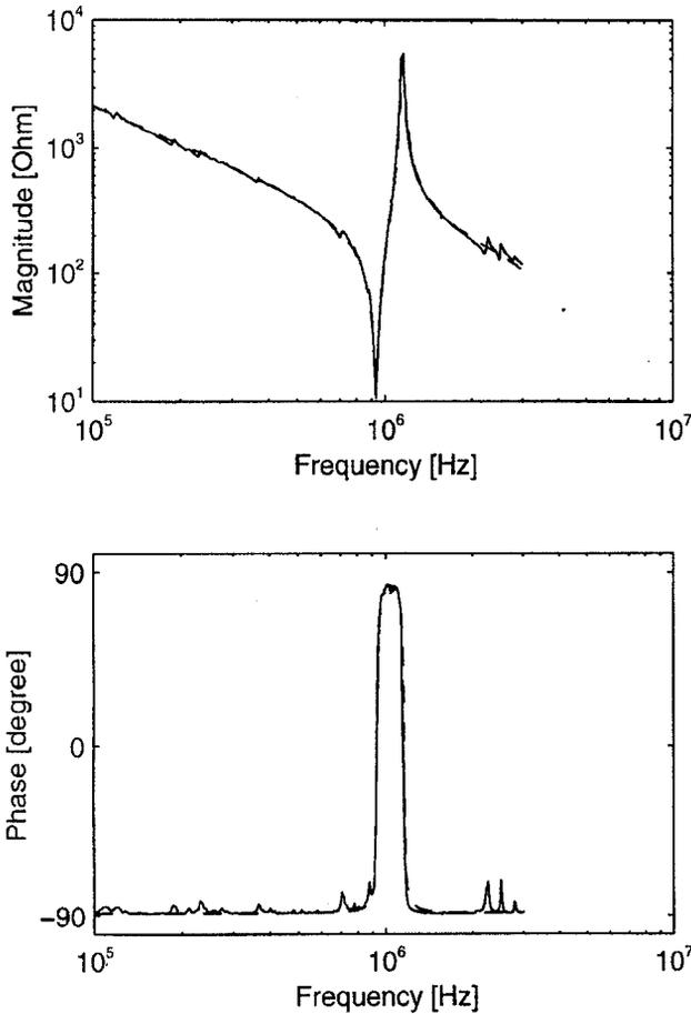
Figure 3: Simulated (-) and measured (·) electrical impedance of the 1:1 by 2 thick aspect ratio PZT-5A pillar, using extracted constants.
