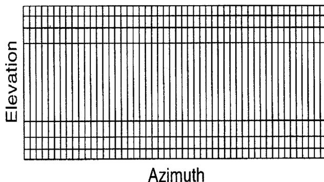
Figure 1: 1.5-D array, illustrating small number of elements along the elevation dimension relative to the azimuth.
