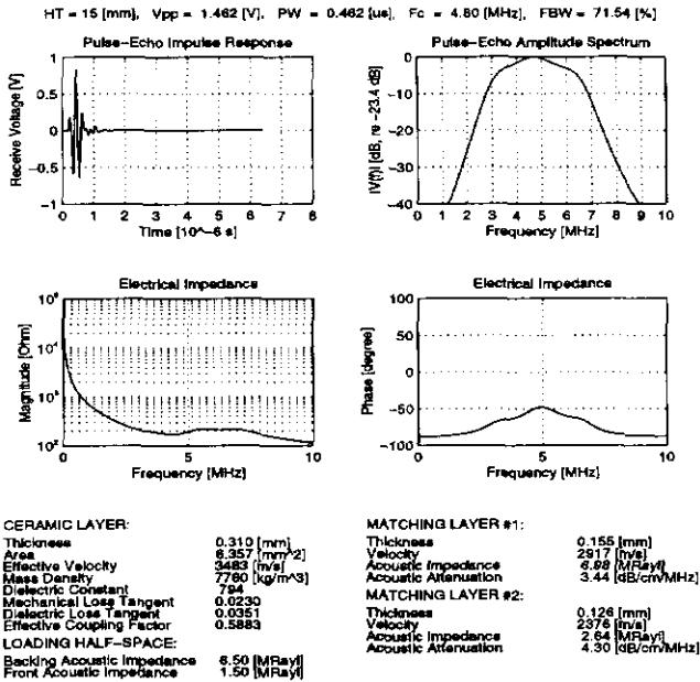
Figure 4: Pulse-echo simulation of a 5 MHz 1.5-D transducer element, using an elevation height of 15 mm.
