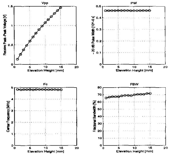
Figure 5: Variation of transducer parameters with elevation height simulated for D-1900 (PZT-5A equivalent) ceramic material.
