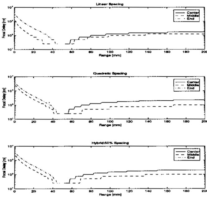
Figure 6: Quantized elevation focal delay versus range for a 15 mm height, 5-element (3 electrical) 1.5-D array. Delay taps are spaced at 25 ns, yet judicious selection of elevation focal zones yields only  $\pm 5$  ns delay quantization error.
