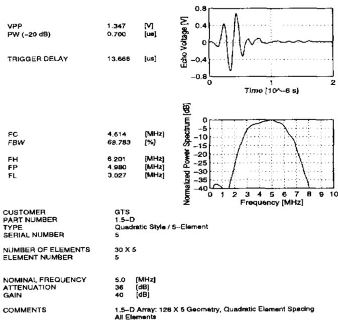
Figure 9: Pulse-echo test results of a 1.5-D array prototype with quadratically spaced elevation. All elements along elevation driven together.
