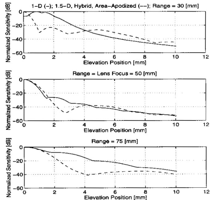
Figure 8: Comparison of elevation beamprofiles of a conventional 1-D array with that of a five element, hybrid spaced, 1.5-D array. The natural apodization resulting from the different transducer element sizes is included. The 1.5-D array is electronically focused at 30, 50, and 75 mm.
