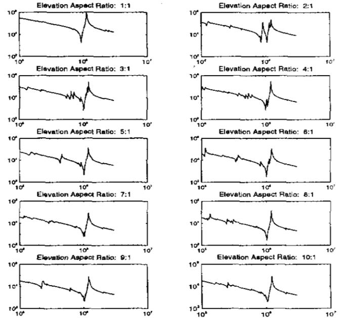
Figure 3: Measured electrical impedance magnitude of parallelepipeds of elevation height to azimuthal width aspect ratios of 1:1 to 10:1, showing asymptotic single mode for 1:1 and 10:1 ratios. The thickness to width aspect ratio in each case is 2:1.
