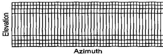
Figure 1: 1.5-D array, illustrating small number of elements along the elevation dimension relative to the azimuth.
