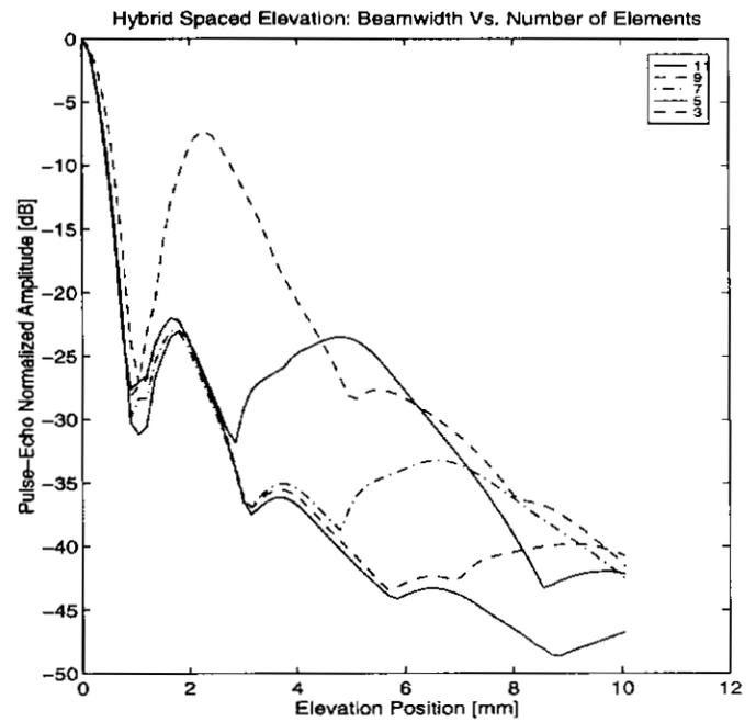
Figure 7: Beamprofile versus element count for hybrid spaced array focused at 3 cm.
