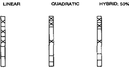
Figure 2: Elevation focusing geometries analyzed, illustrating a five (5) elevation element array. Exploiting symmetry, consecutive outer pairs of elements are electrically connected for on-axis focusing, resulting in less hardware.
